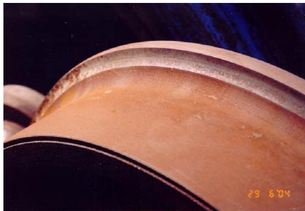
Figure 4 - An unacceptable witness mark
