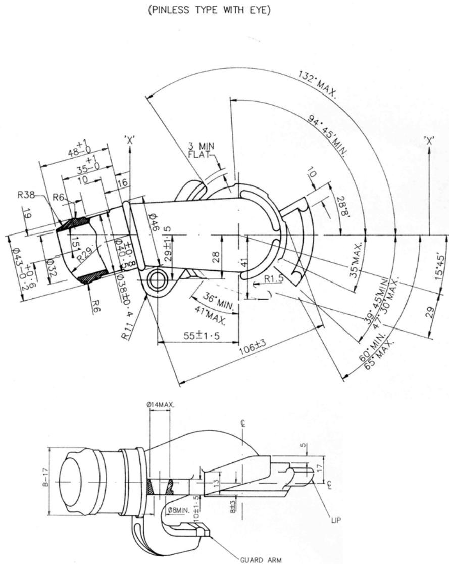
Figure 7 - Air brake coupling hose head
