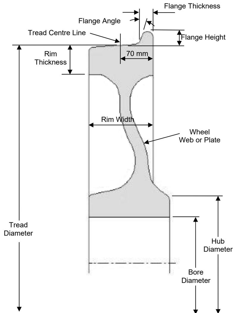
**Figure 1 – Wheel parts and principal dimensions**
