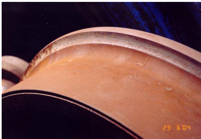
Figure 4 - An unacceptable witness mark
