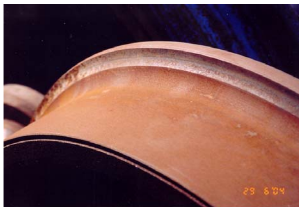
Figure 15 - An unacceptable witness mark
