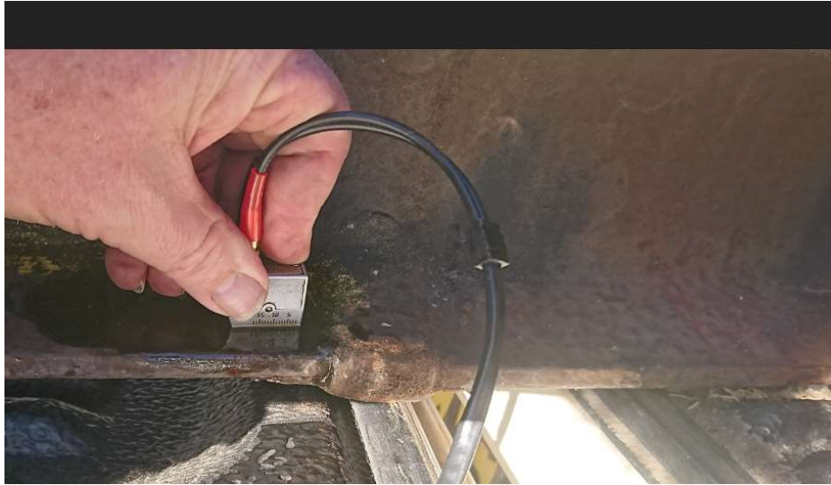
Figure 9 – Photo of correct orientation mini 70 toward weld
