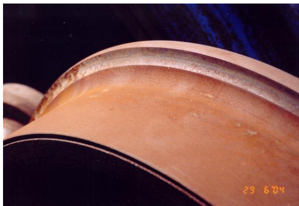
Figure 15 - An unacceptable witness mark
