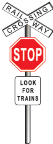
FIGURE 8: Type D level crossing STOP sign
