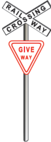
FIGURE 7: Type B level crossing GIVE WAY sign
