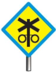
FIGURE 4: Trackside sign before standard Type F level crossing with predictor
